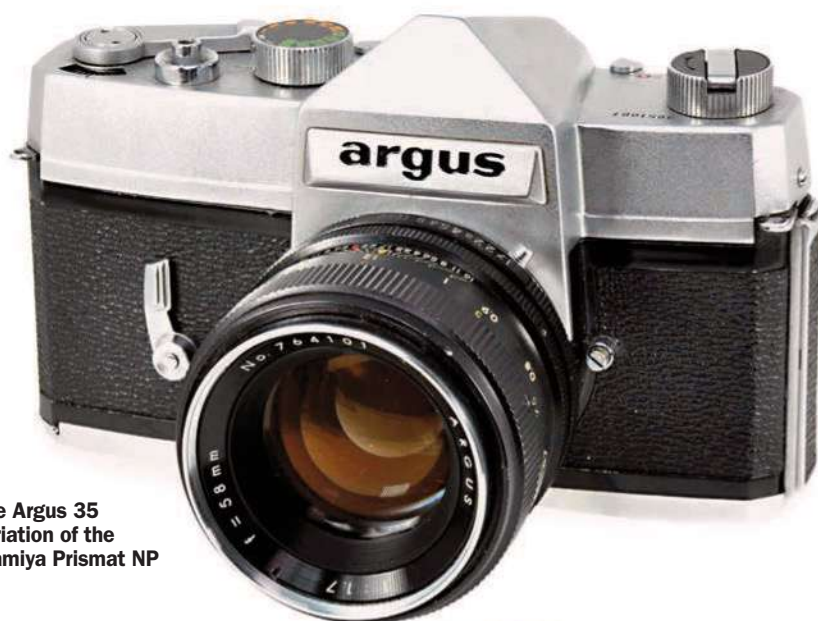
The Exakta-influenced lens mount and aperture stop-down coupling used on the Prisma NP
