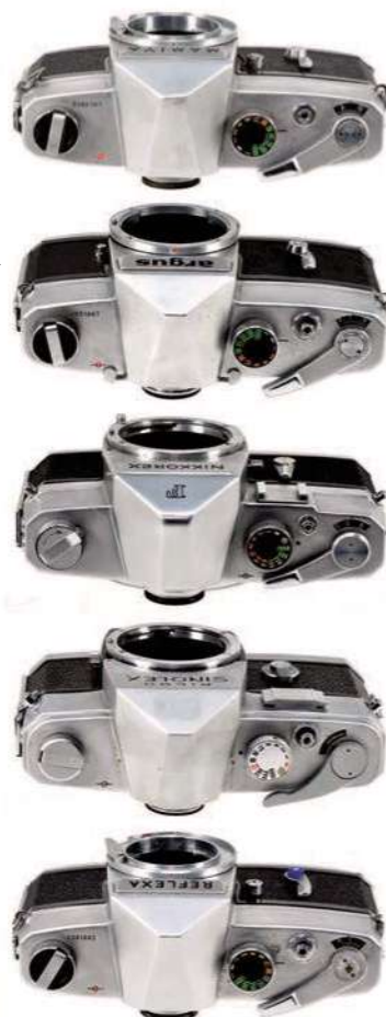
The similarity in top plates on the five cameras, top to bottom: Mamiya Prisma NP, Argus 35, Nikkorex F, Ricoh Singlex and Reflexa
